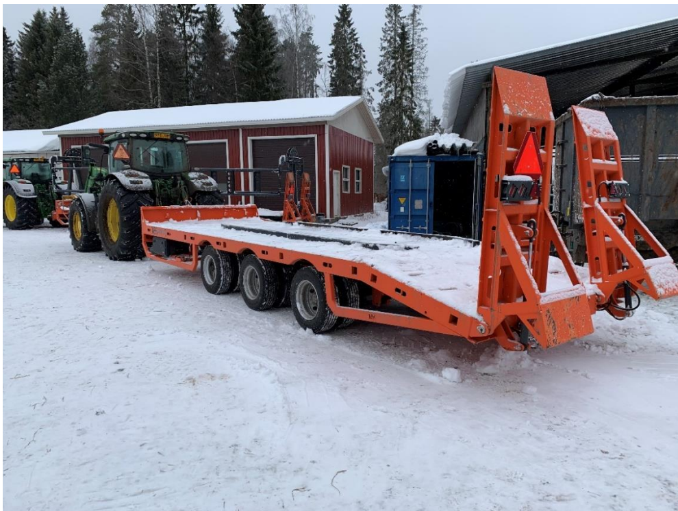
Picture 4. MPH Trailer 30 for earthmoving machine transportations.
