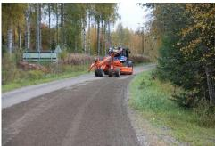
Picture 7. Start-up and end-up phases are need to enter systematically, so that moved material do not give height difference. When Grader is put to a transport position or dismantle machine, replacement valve should be used to get wings to a narrow position.
