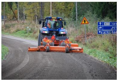
Picture 1. MPH Grader 5.3 with road options are maintaing sandy road in Heinävesi area.
