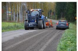
Picture 6. When road maintenance works are done for public roads, other traffic must be observed. The facing traffic gives a road so that the operation runs smoothly. Wing extension of Stone collector has been lifted up to give more space for facing traffic.
