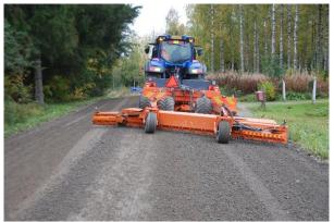
Picture 4. Stone collector has floating assembly and 10 cm movement allowance to machine body. Stone collector moves on its own wheels, but hydraulic adjustment in inner wheel could help height adjustment. The additional wing on the end of Stone collector on the ditch side moves hydraulically.
