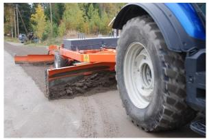
Picture 5. Petri's MPH Grader 5.3 has four pcs of extra weights, about 1600 kg. Basic MPH Grader 5.3 weights about 2000 kg. MPG Grader 5.3 field version has 2x400 kg extra weights, when the total weight is 2800 kg.
