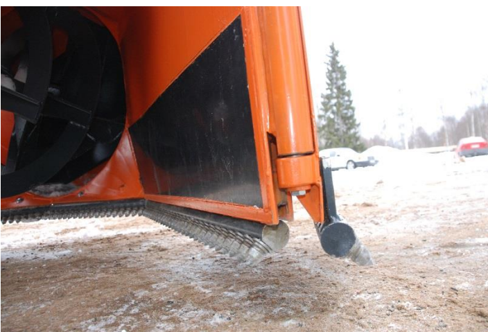
Picture 7. MPH Snow Blower has plastic in the side structures and this makes sliding of snow very effective. The snow is transferred by spiral impeller to the mouth and throwing impeller are solid.
